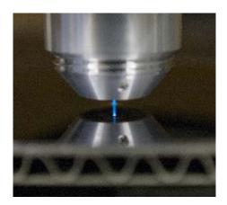
Coating through cathodic evaporation at atmospheric pressure
